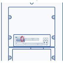
c. Click in SD card as on the right side of main module as below, and with a beep means the door station is in updating, end with 2 beeps means the update is finish.
